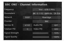
4 Adjust your antenna so that the two specifications **signal strength** and **signal quality** display a preferably high value.
